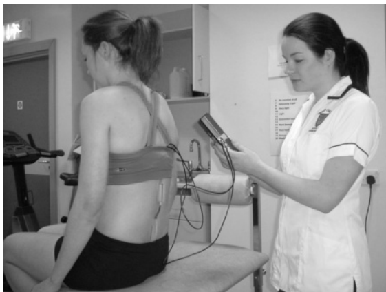
Figure 6.9 Assessment of repositioning skill using an electrogoniometer.
