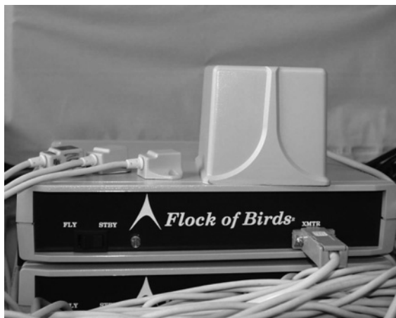
Figure 3.3 The Flock of Birds™, an electromagnetic motion tracking system. Reproduced with kind permission from Ascension Technology, Vermont, USA.
